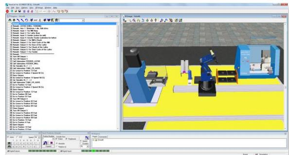
Students utilize the offline capabilities of RoboCell 3D graphic simulation software to design, program and execute an unlimited number of simulated industrial applications and gain maximum hands-on training experience.
